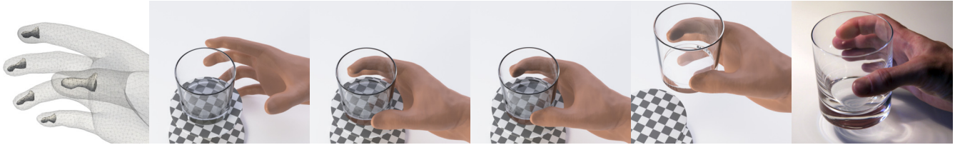
Fig. 1. A rigid whiskey glass is pinched between the index finger and thumb of an animated hand model and lifted up. The first frame shows the internal geometry of the distal phalanges whose vertices drive the finger tips of the tetrahedral simulation mesh of the hand. The remaining hand bones and tendons (not shown) are used to determine other interior animated vertices. The following frames show a selection of frames from the resulting simulation showing the grasp, lift and hold of the glass. The last image shows a photo of a similar scenario for reference. The collision surface of the hand is represented by an implicit function approximating a smoothed distance potential, while the glass surface is sampled using discrete points. Our method produces realistic deformation at the point of contact between the fingers and the rigid object.
