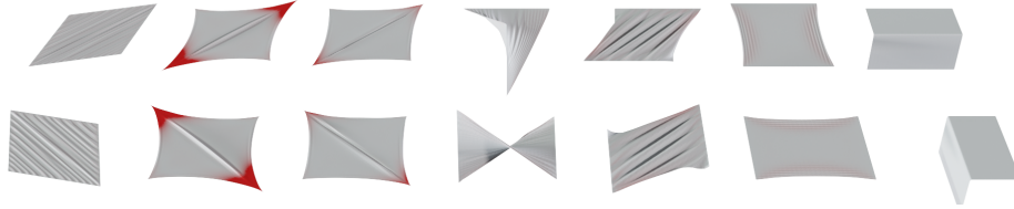
Figure 5.11: Re-simulation with the estimation of Houdini’s silk pre-set. The square cloth swatch is re-simulated using the estimated parameters using our XPBD solver. The set of targets used during optimization (training set) includes configurations from columns 2, 3 and 7. The vertex displacement error is color-coded in red with a maximum set to 2 mm. In the second column, errors are clustered on the large stretch areas with a maximum of 6 mm while it is below 2.4 mm in the remaining columns.
