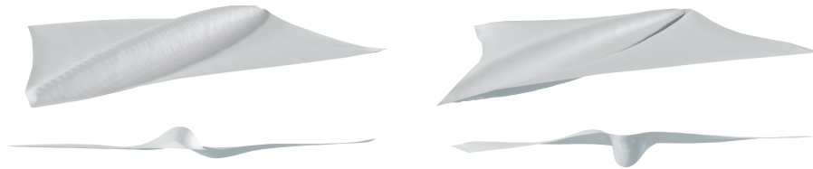
Figure 5.4: Wrinkle bifurcation: two valid cloth configurations with contrary wrinkle patterns shown from above (top) and side (bottom). The same cloth swatch is pulled with the same force at opposite corners.
