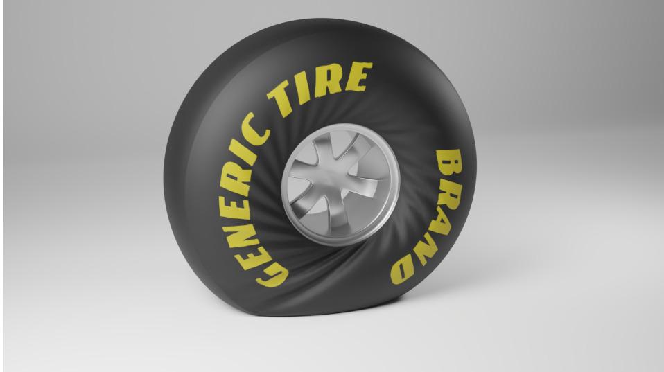
Figure 4.12: Dragster tire wrinkle. A soft tire spins against the ground with a large friction coefficient, causing the rubber to wrinkle.
